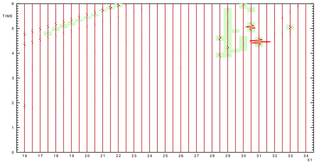
Figure 28: Born (red) and ray-theory (black) seismograms computed in model P1-3-10% using no amplitude cut-off.
