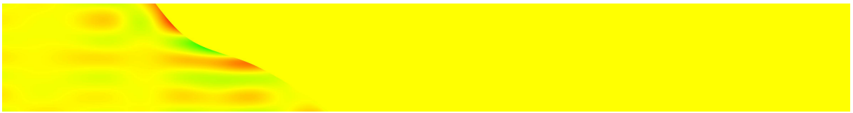
Figure 2: P-wave velocity perturbation between model P1-1-10% and the background model. Positive perturbations are red, negative perturbations are green. Zero perturbations are yellow.
