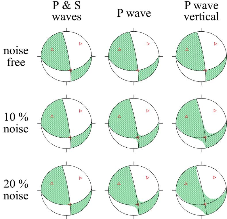
**Figure 4:** Synthetic experiment of moment tensor inversion using correct velocity model for calculation of responses of the medium. Upper row – noise free input data, middle row – random noise up to 10% of maximum amplitude added to the input data, bottom row – random noise up to 20% of maximum amplitude added to the input data. Columns from left to right: inversion of P together with S wave amplitude, inversion of P wave amplitude, inversion of vertical P wave amplitude only.
