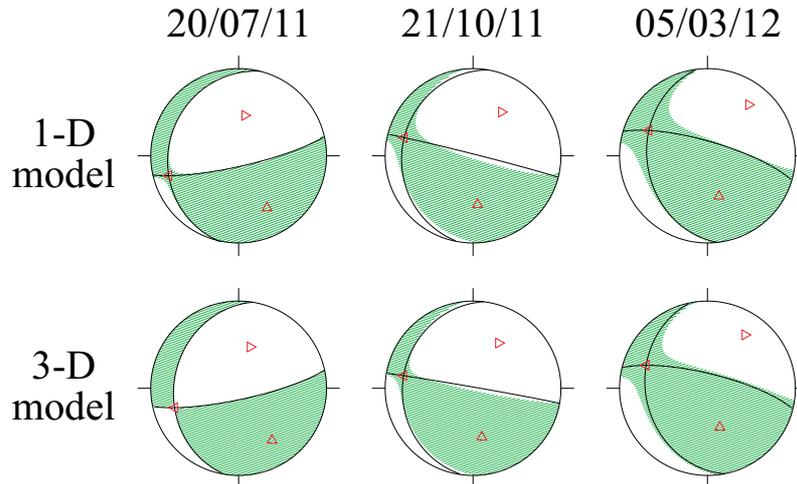
**Figure 6:** Moment tensor inversion of sample events from Dobrá Voda. Upper row – 1-D model used for calculation of responses of the medium, bottom row – 3-D model used for calculation of responses of the medium. Each column represents different seismic event from the mountain region of Malé Karpaty.
