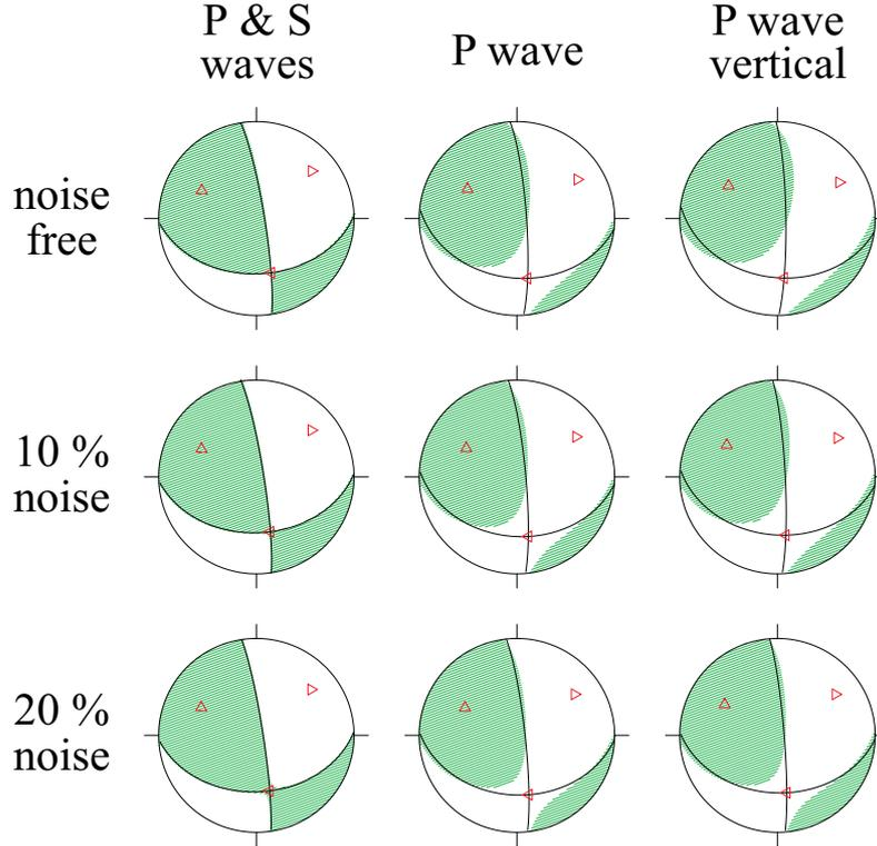
**Figure 5:** Synthetic experiment of moment tensor inversion using incorrect velocity model: 1-D model for calculation of responses of the medium, while the synthetic data correspond to 3-D model. For details see caption of Figure 4.
