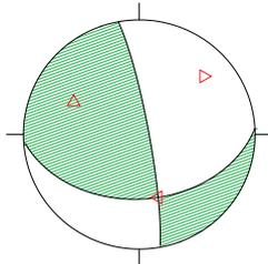
**Figure 3:** Source model of tectonic event for synthetic experiment. The mechanism in traditional fault plane solution, i.e. equal area projection of the lower hemisphere; black lines - nodal lines of the DC part; triangle up - T axis, triangle right - P axis, triangle left - N axis; green zone - compressions.
