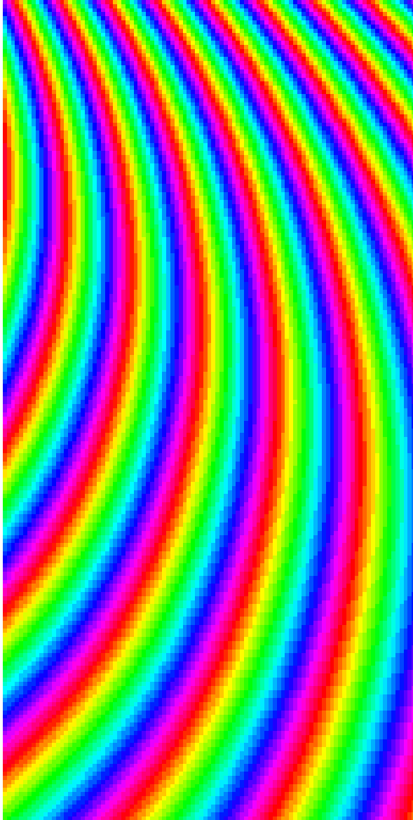
Figure 1. The real part of travel time corresponding to the point source located at x^1 = 0.000 km, x^3 = 0.000 km in the complex-valued velocity model with velocity (1 - i0.05)\text{km s}^{-1} at the top and (3 - i0.00)\text{km s}^{-1} at the bottom. The values of the real part of travel time range from 0.440 s to 0.880 s. The colour circle corresponds to the time increment of 0.050 s. The yellow colour corresponds to values 0.450 s, 0.500 s, 0.550 s, etc. The maximum absolute error of the numerical solution is 1.3 \times 10^{-6} s.
